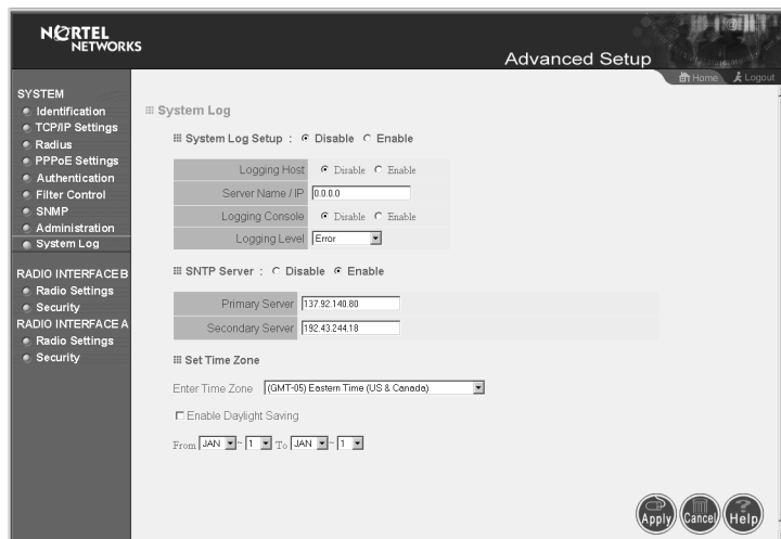
Figure 6 SNTP Server enabled
