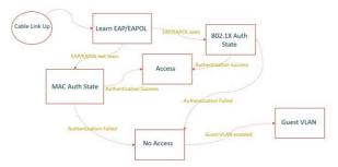
Note: If enabling 802.1X on the end-station, a port bounce on the ISW will be required to perform 802.1X authentication.
