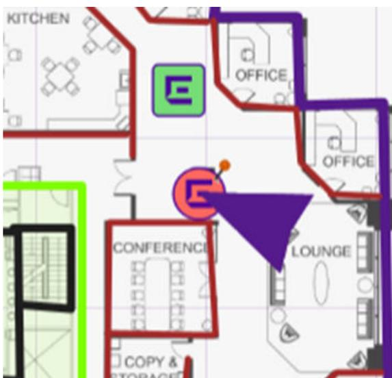
**Figure 25: Configuring the AP Camera Angle Towards a Doorway**
