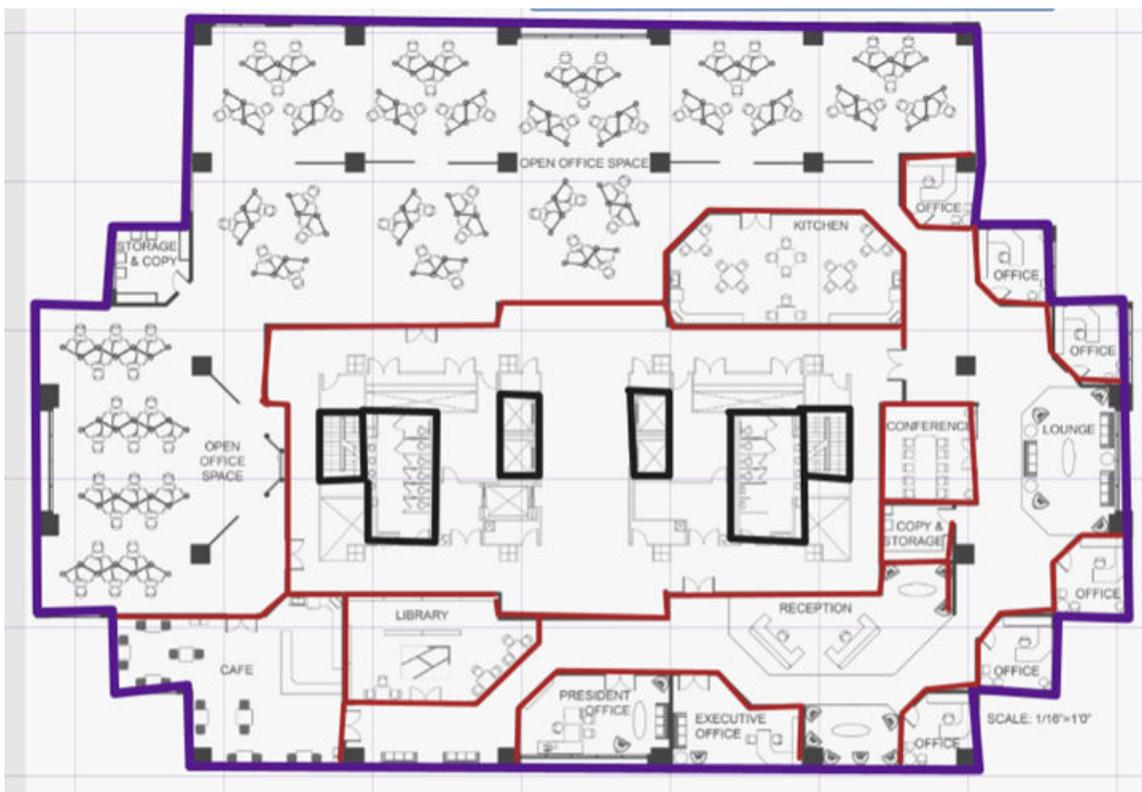
**Figure 17: Inner Walls Drawn for Concrete and Drywall**
