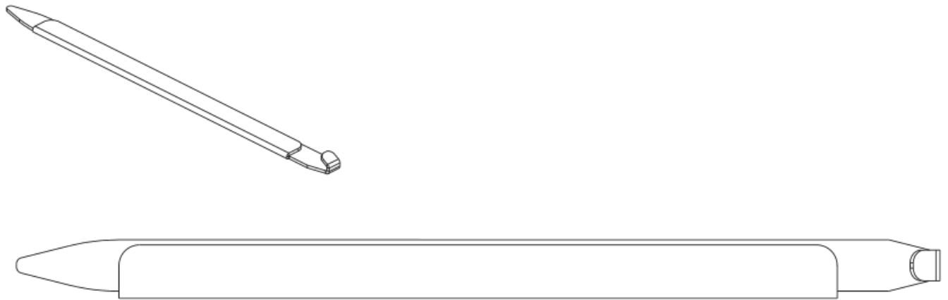
FIGURE 61 Optical transceiver extraction tool
