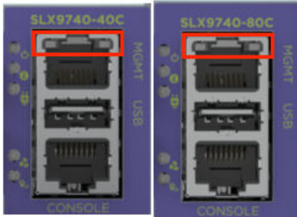
Figure 32: RJ45 Management Port LEDs
