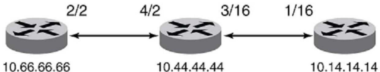
FIGURE 27 Inbound FEC filtering example
