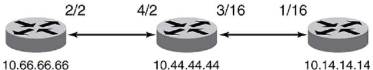
FIGURE 27 Inbound FEC filtering example
