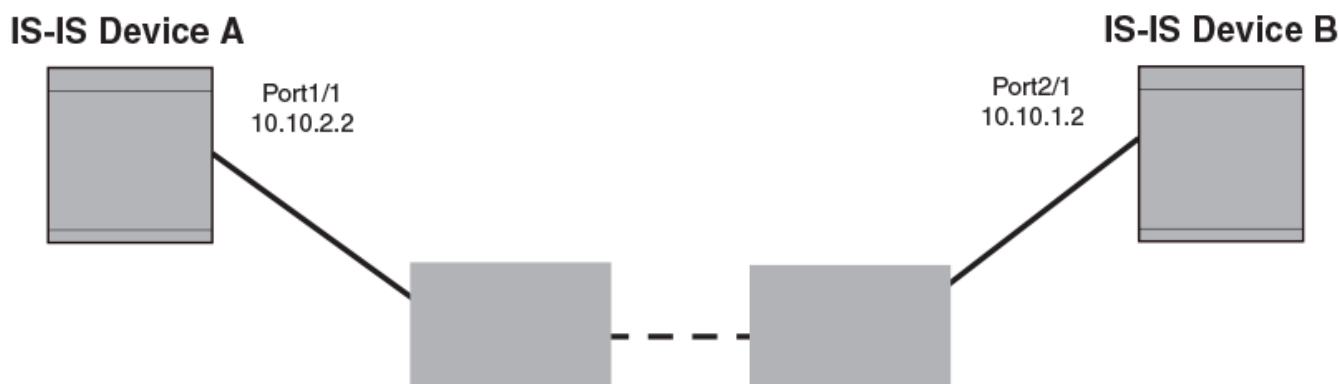
Figure 44: IS-IS Point-to-Point configuration
