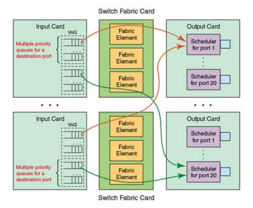
Figure 3: QoS for unicast traffic
