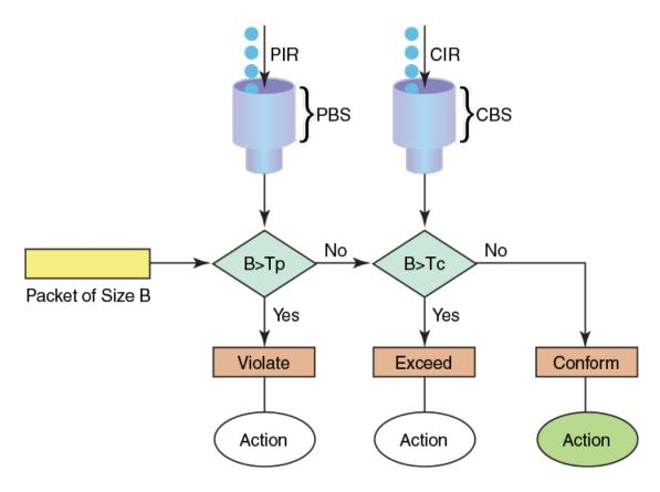
Figure 2: Two-rate, three-color marker
