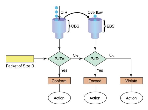
Figure 1: Single rate three color marker
