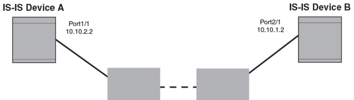
Figure 43: IS-IS Point-to-Point configuration
