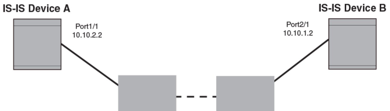
Figure 45: IS-IS Point-to-Point configuration
