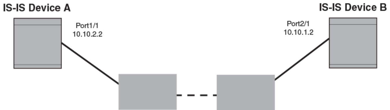
Figure 45: IS-IS Point-to-Point configuration
