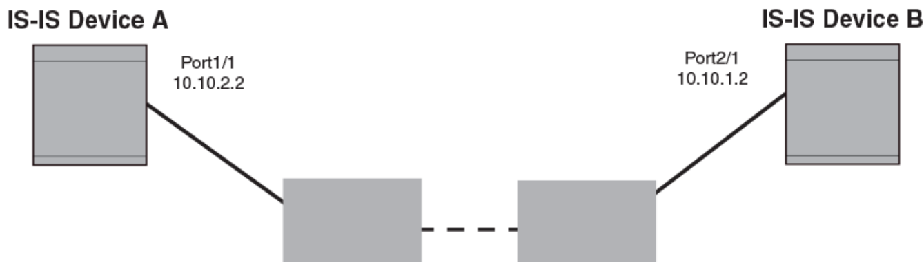
Figure 45: IS-IS Point-to-Point configuration
