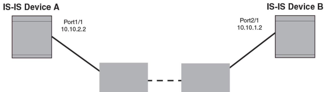
Figure 46: IS-IS Point-to-Point configuration
