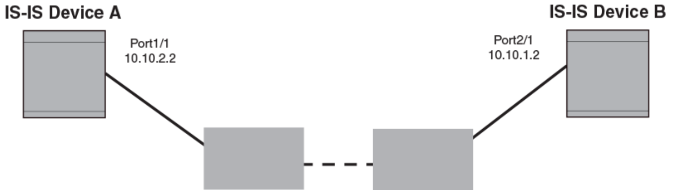
Figure 52: IS-IS Point-to-Point configuration
