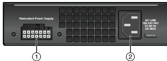
Figure 192: Power Connectors on STK-RPS-150PS (rear view)
