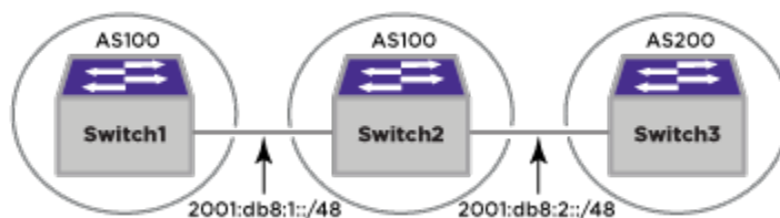
Figure 256: BGP IPv6 Example
