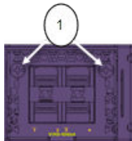
Figure 36: Tighten Screws on the Inserted VIM5 Module
