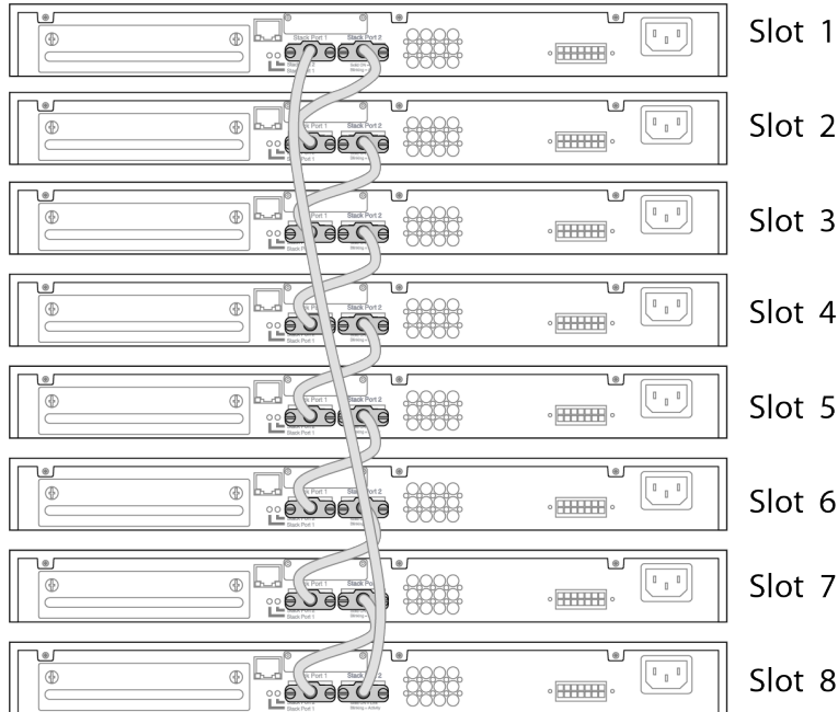
Figure 10: SummitStack Cable Connections Using Eight Switches with Integrated SummitStack Ports
