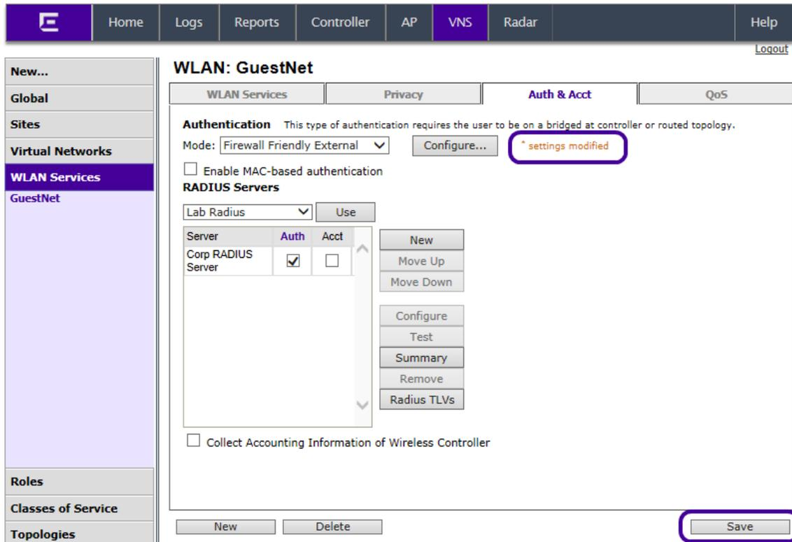
Figure 21: Saving the WLAN Service
