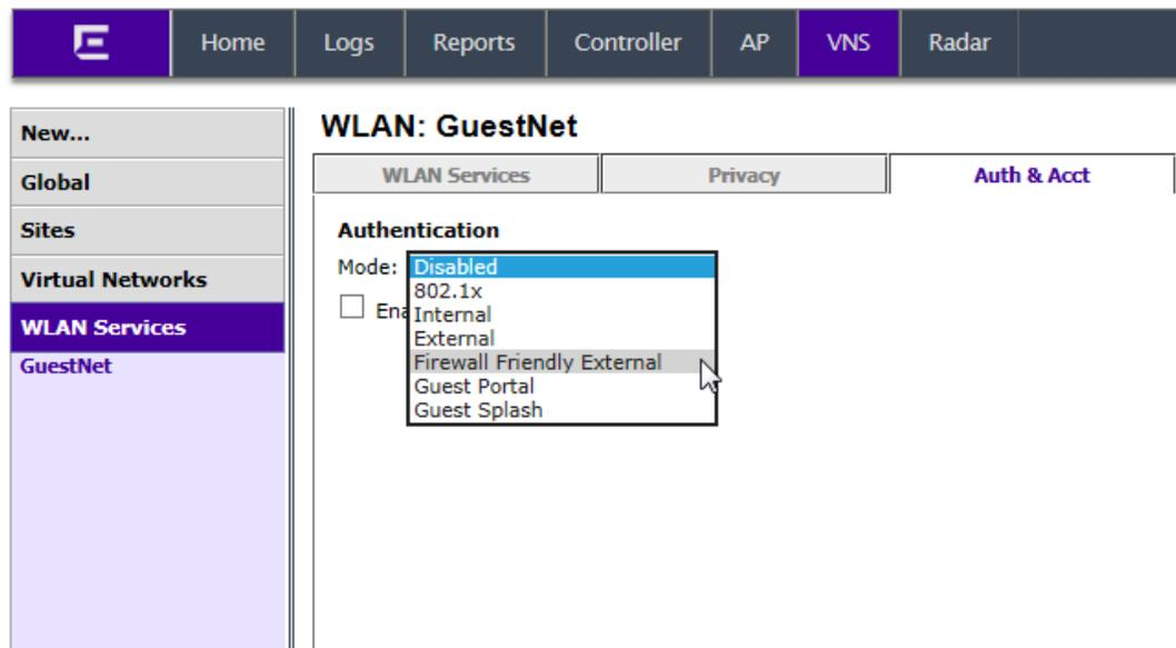
**Figure 18: Selecting the “Firewall Friendly External” Support Option**
