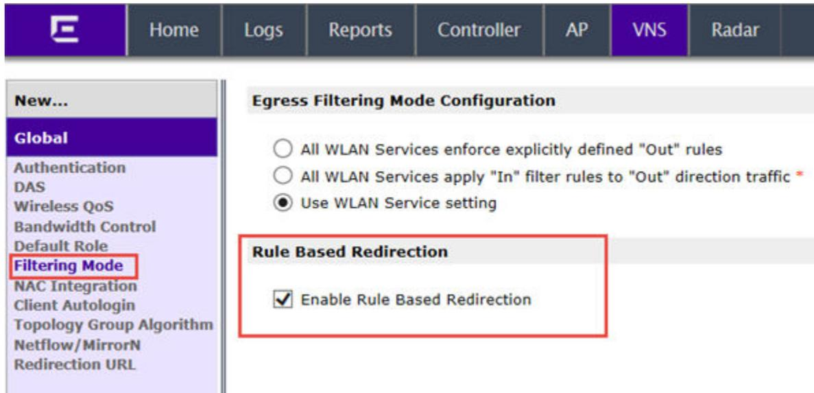
**Figure 6: Enabling Rule-based Redirection**
