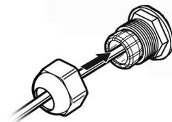
7. Tighten the adapter assembly by hand to 5-in. lbs.
