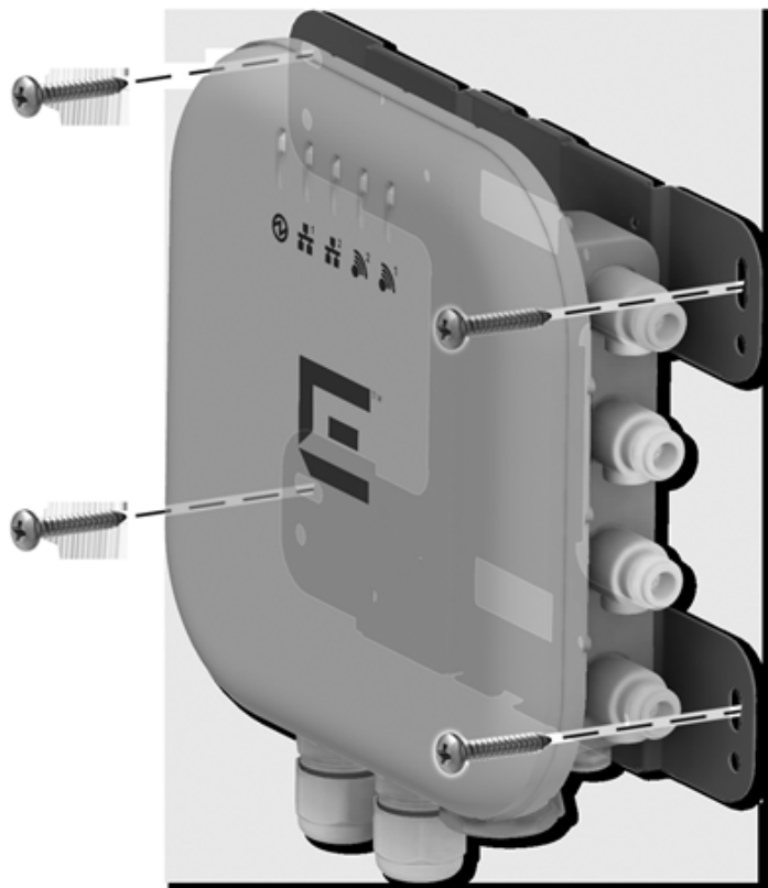
Figure 4: Mounting the AP3965 to a Wall
