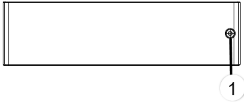
Figure 15: Plastic service panel top captive screw
