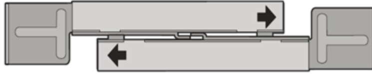
Figure 6: Bracket halves attachment procedure
