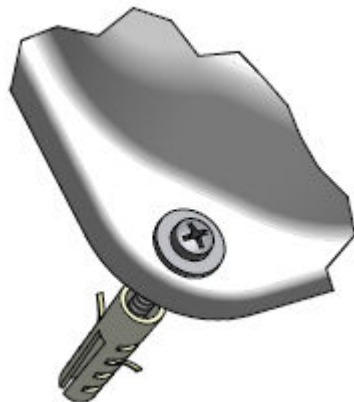
Figure 178: Self tapping screws inserted into the plastic wall insert plugs
