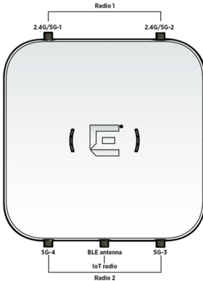
Figure 8: AP310e access point external antenna connector ports
