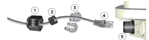
Figure 7 Weatherproof Ethernet cable housing
