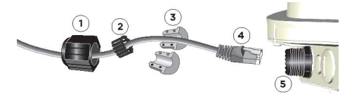
Figure 7 Weatherproof Ethernet cable housing
